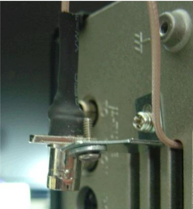
STEP 2: Connect the softrock. The antenna input of the softrock will attach to the IF-2000 BNC dongle on the back of your rig. Power can be supplied from the DC jack on the back of the rig. And the computer sound card will connect to the audio output of the SDR.
