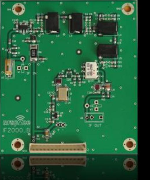
It's advertised to work on the FT950 as well. It converts the 69.55 Mhz 1<sup>st</sup> IF down to a 10.55 Mhz intermediate IF output which terminates in a BNC pigtail that hangs out of the back of the FT2000. No permanent modifications to the FT2000 are involved as it occupies the same location as the DMU bandscope card does (see red arrow pointing to the IF2000 card in the pic below).
