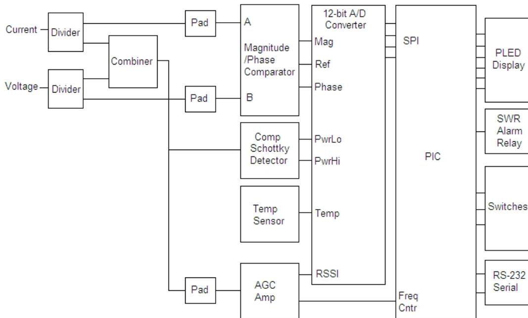
First, instead of using a coupler that produces forward and reflected power signals, the LP-100 uses a pair of transformers that sample current in the transmission line and voltage across the load. The samples are split into two paths, which provide signals to both the gain/phase comparator and the power detector.
