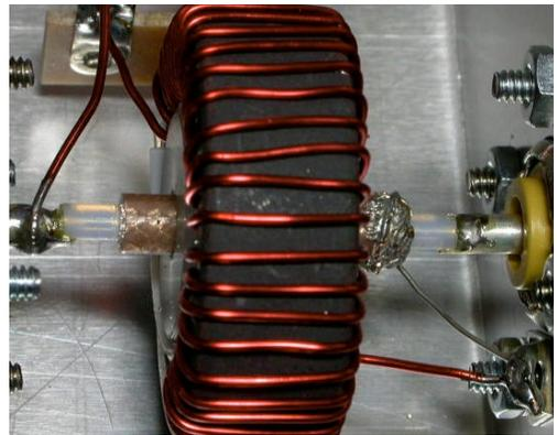
Refer to the drawing and pictures during assembly of the coupler. The top picture is courtesy of Dario, N5QVF, and the lower right one is courtesy of Stan, W5EWA. The sequence of pictures below is from Jack K8ZOA. Jack developed a clever way to ensure proper winding of the cores, both for spacing and coverage of the windings. Details of Jack's winding methodology is found below.
