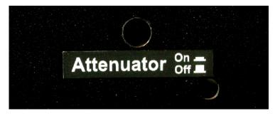
Install the front panel decal next. You can choose to place it either above or below the hole. Just peel it off the blue backing and carefully place it on the front panel. A tweezers might be helpful for this task.
