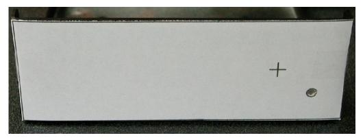
Once aligned, tape the template in place and use a center punch to mark the hole center. Then use a 7/32" drill or punch set to create the hole. For users in metric countries I would recommend a 5.6mm bit if available, otherwise you could try 5.5mm, although it might be a bit tight and need to be filed. 6mm is probably too loose. Be careful not to scratch the faceplate while drilling / punching the hole. Masking tape helps with this.
